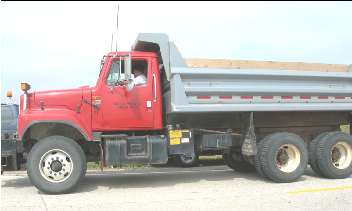
Figure A.12. Loaded truck for strain testing
