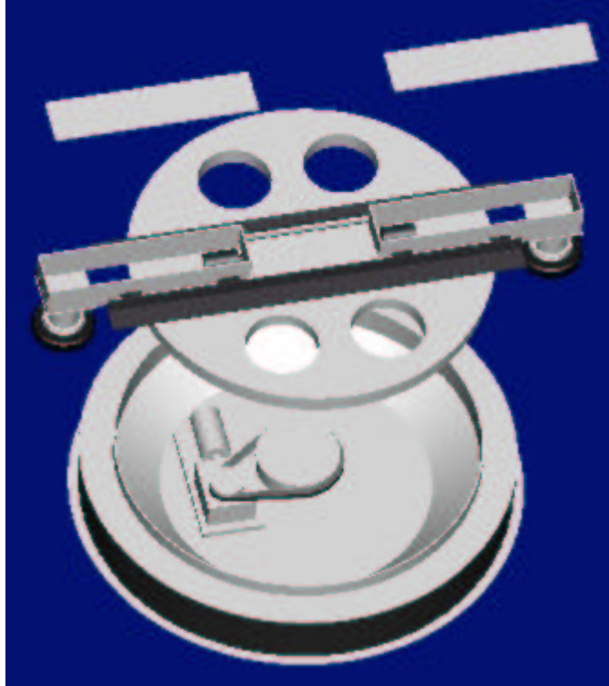
Figure 3: Schematic drawing showing interior assembly of TPTA
