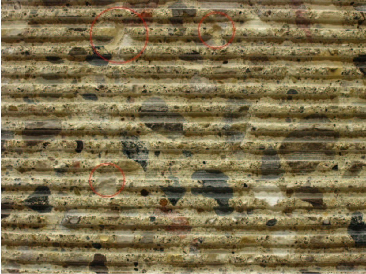
Figure 17: Broken fins on TI 2-2. Red circles indicate examples of points where ridges have broken off, leaving a rougher contact patch
