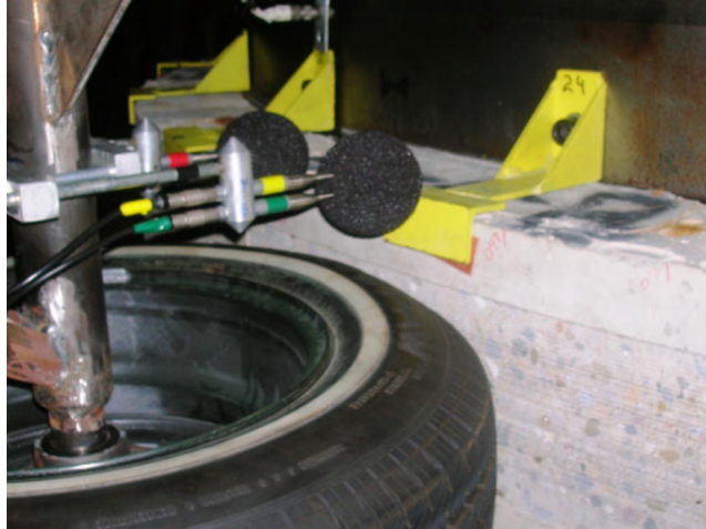
Figure 4: Placement of on-board sound intensity probes in relation to test tire and sample
