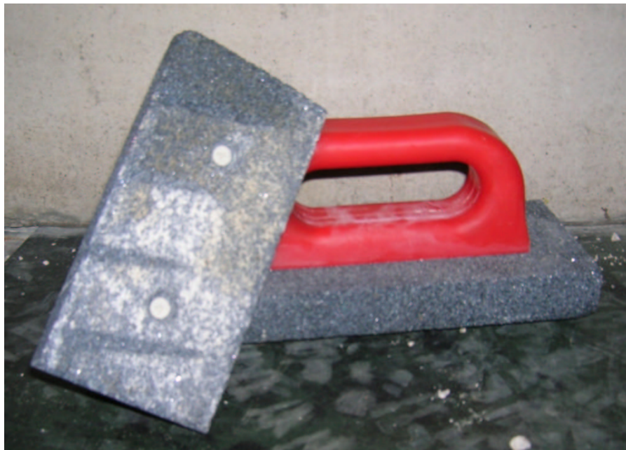
Figure 7: Abrasive blocks used to wear down fins on fin wear investigation samples
