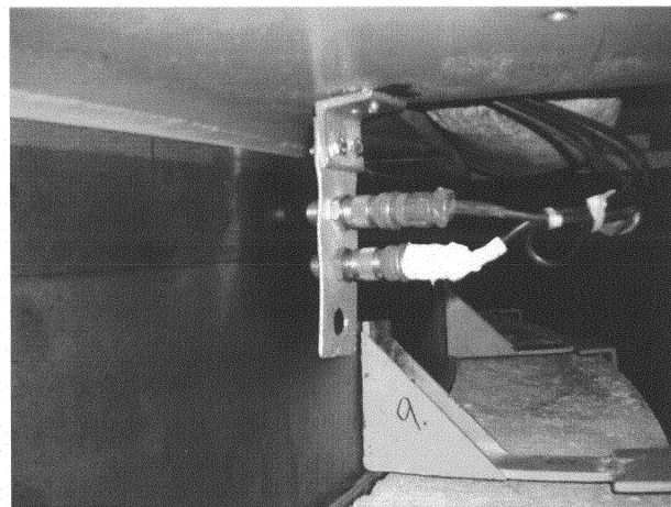
Figure 5: Magnetic triggers attached near test tire on TPTA
