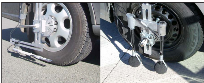
Figure 2. Comparison of GM (left photo) and ACPA (right photo) OBSI Equipment
