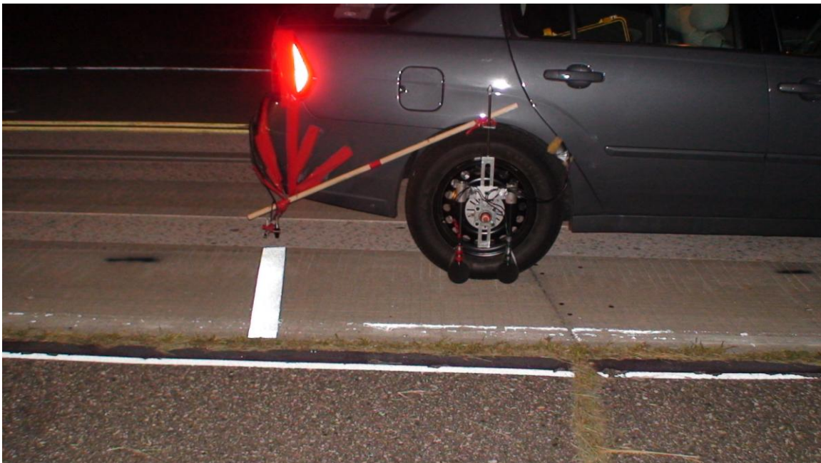
Figure 13 Side View of OBSI Equipment and Laser Trigger Suspended from Vehicle
