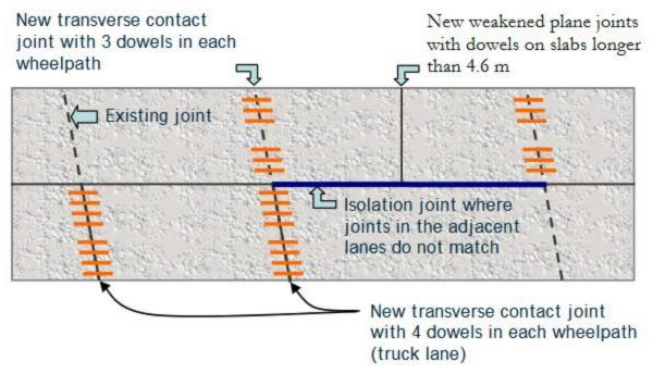
Figure 13. Plan showing number of dowel bars per joint in California. (Caltrans Slab Replacement Guidelines, 2004). Note that perpendicular joints are used with dowels.
