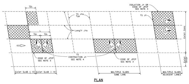
Figure 14. Plan showing individual slab replacement in California. (Caltrans Standard Plans, P8, 2015).
