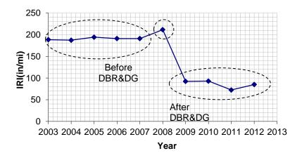
Figure 9. Texas US 69 JPCP diamond grinding (52% reduction).
