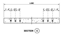
Figure 5. Washington State DOT DBR design and layout diagram for skewed joints. (Washington State DOT Standard Plan for DBR, A-60.20-03)
