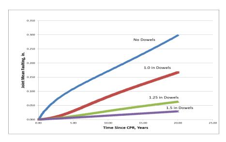
Figure 3. AASHTOWare Pavement ME Design example output for a JPCP CPR grinding project, with and without DBR.
