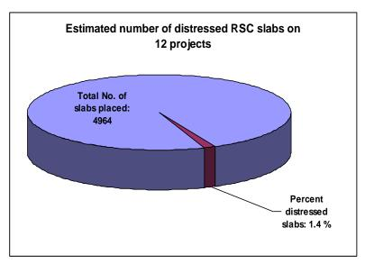
Figure 23. Percent distressed slabs on 12 surveyed RSC projects in California.
