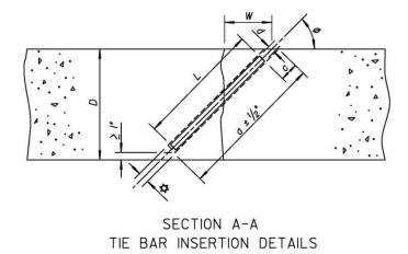
$\clubsuit$  Drill diameter will be not less than  $\frac{1}{4}$  larger than the tie bar diameter and no more than  $\frac{3}{4}$  larger than the tie bar diameter.
