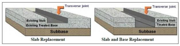
Figure 12. Slab and base replacement. (Caltrans Concrete Pavement Guide, 2015)
