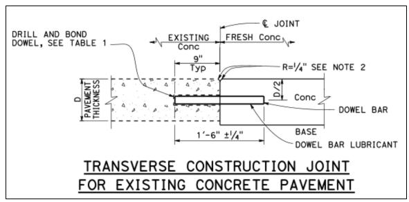
Figure 19. Dowel bar anchoring in California. (Caltrans Standard Plans, P10, 2015)
