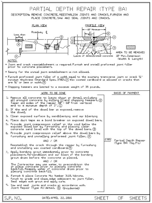
Figure 26. Minnesota PDR BA diagram for milling. (MnDOT, 2017)
