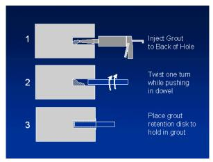
Figure 21. Illustration of recommended procedure to anchor dowels securely into face of slab.
