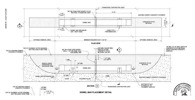
Figure 6. Washington State DOT DBR placement detail. (Washington State DOT Standard Plan for DBR, A-60.20-03)
