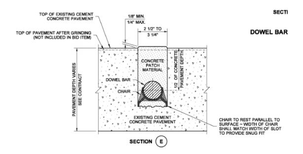
Figure 7. Washington State DOT DBR cross-section layout diagram. (Washington State DOT Standard Plan for DBR, A-60.20-03)
