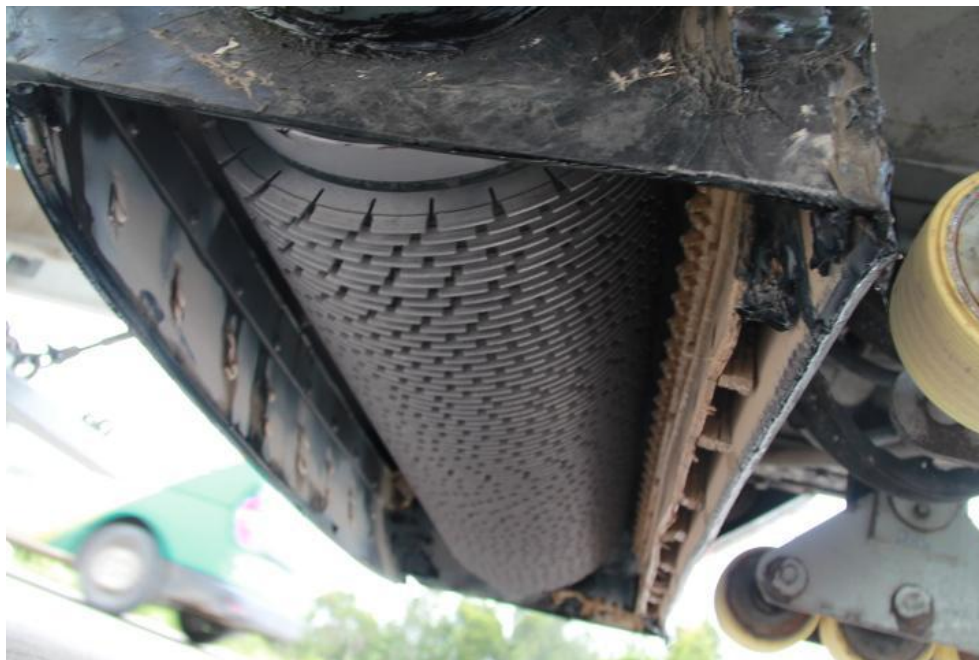
Figure 8: View of the suction devices (to the right of the drum) to collect the slurry from the concrete surface
