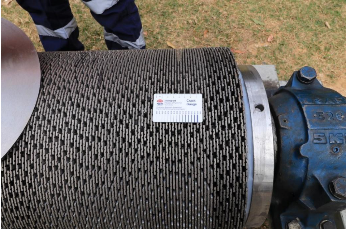
Figure 6: View of the grinding drum with the blades spaced 2.54 mm apart
