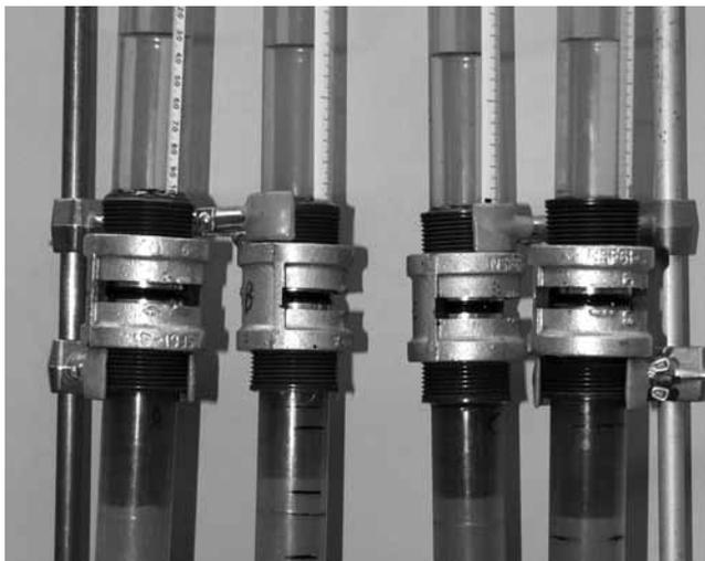
Fig. 1. Infiltration progress in four 2.5-cm-diameter soil columns as used in this study.
